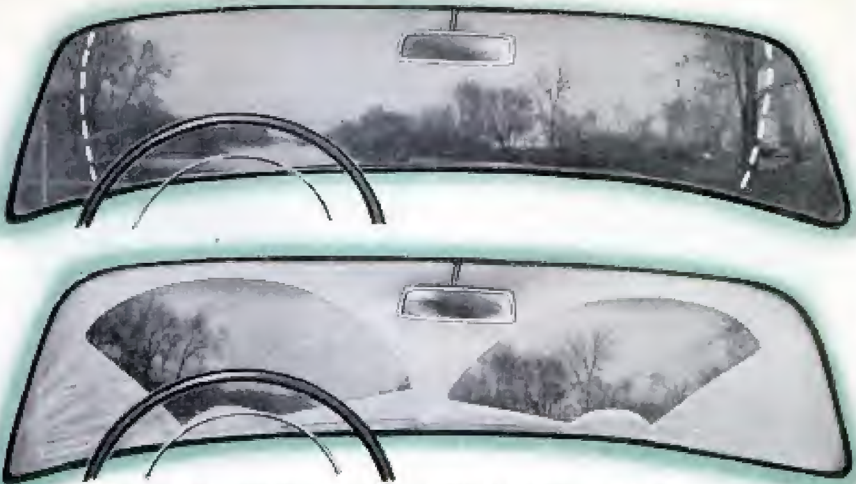
Vision through wrap-around windshield is great. Dotted lines show usual windshield outline. But when covered by snow or mud, glass has large blind areas as lower photograph shows
